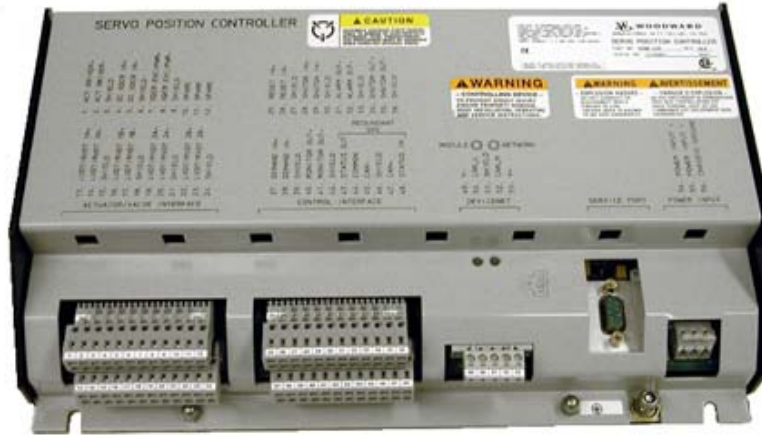
Figure 2-10. Servo Position Controller
